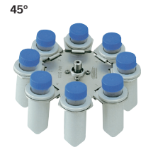
Swing-out rotor, 8-place, for 8 x 50/15 ml Falcon tubes n = 4,000 \text{ min}^{-1} , RCF 2,469 stainless steel, with suspensions, aluminium.
