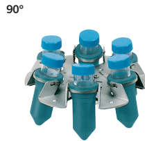
Swing-out rotor, 6-place, for 6 x 50/15 ml Falcon tubes n = 4,000 \text{ min}^{-1} , RCF 2,701, Stainless steel, with suspensions, PA, fiberglass reinforced.
