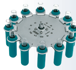
Swing-out rotor, 12-place, for 12 x 15 ml n = 4,000 \text{ min}^{-1} , RCF 2,683, Stainless steel, with suspensions No. 01621, PA, fiberglass rein- forced.
