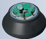
Angle rotor, Cat. No. 01556 6-place, n = 9,000 \text{ min}^{-1} , max. RCF 10,595
